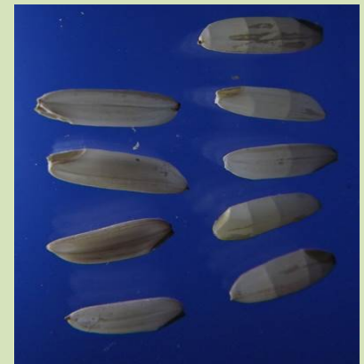
Rice kernels with internal fissures (right side of photo) are more likely to break during the milling process than intact kernels (left). Fissure resistance reduces breakage during milling which
